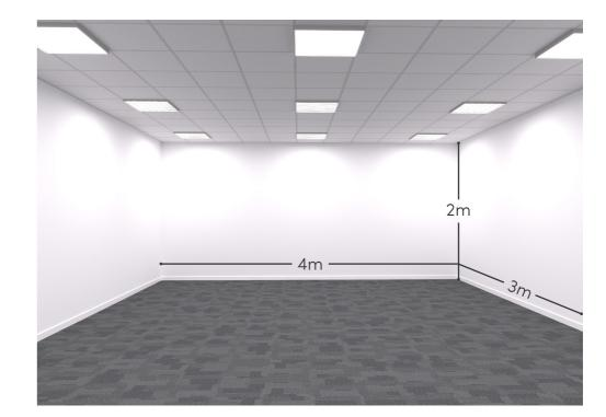
The above dimensioned room without any Eden sound absorbing tiles will have a reverberation time of 1.0 second (the reverberation time is defined as the length of time required for sound to decay 60 decibels from it's initial level).
