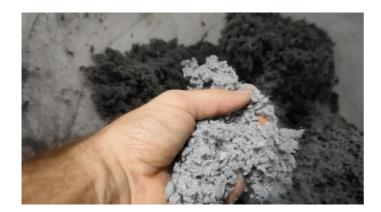
The material is shredded into small pieces prior to chemical processing.
